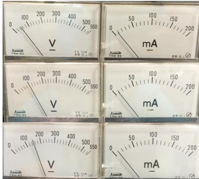
Figure 2-12 Substrate bias power supply panel of 50, 100, 150 V.
